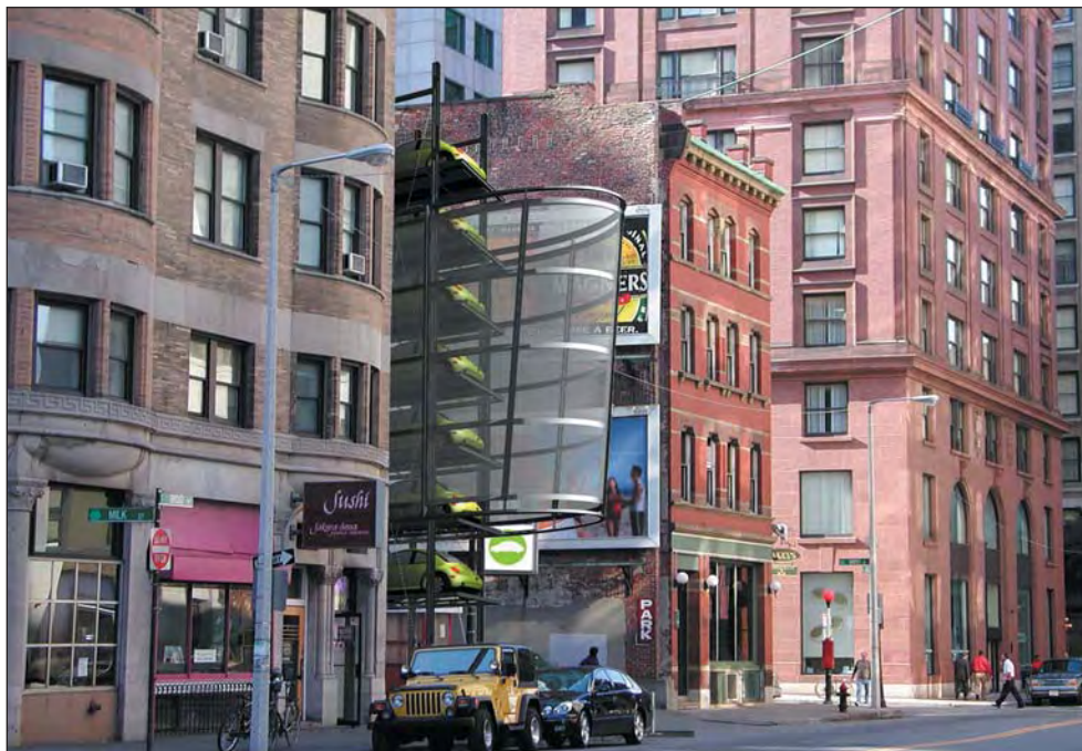
This design by Boston-based Moskow Architects for a Zipcar Dispenser in the city, which would stack cars in mechanisms above unused alleys while employing the machinery's scrim-like designed surface for advertising, is one of six winners the Boston Society of Architects' Unbuilt Architecture Design Award.
